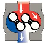
As the impellers continue to turn, the volume of gas in the left cavity is discharged. Simultaneously, gas is entering the space between the right impeller and housing.
